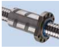
■ Series 1416: DIN standard flanged nut, ball oversize preload
